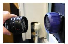
A single multipin connector allows the operator console to be disconnected via one reliable plug and socket.
