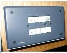
The Kramer RC8IR touch panel providing network, RS-232 and IR control to simplify projector and plasma screen operation
