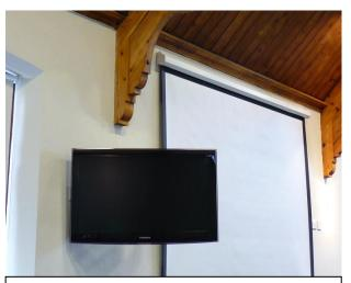
Picture showing one of the wall mounted LCD displays mounted on a Z-bracket for angling to different areas of the congregation depending on room orientation. Via a custom designed four-output PC, every display has the option of showing either the main projection information, working screen or desktop as preferred.
